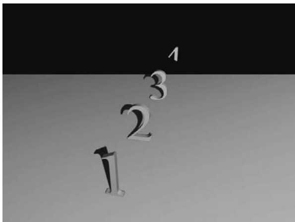
Figure 11.18 A far clipping plane cuts off the distant extents of a scene.
