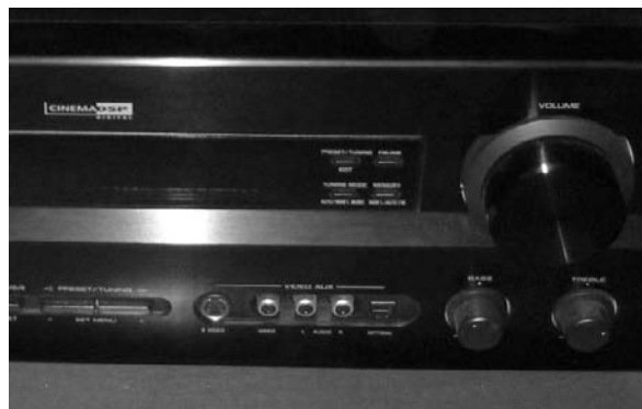
Figure 1.3 A raster image does not scale up very well. Here is the front of a stereo receiver that has been blown up by several hundred percent. The pixels look blocky.
